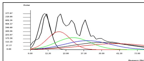
Figure 3: Spectral decomposition for reservoir interval. The color of the frequency distribution curve indicates the RGB component for the color blend. The frequency magnitude of the shallow section is the black curve displayed in background.
