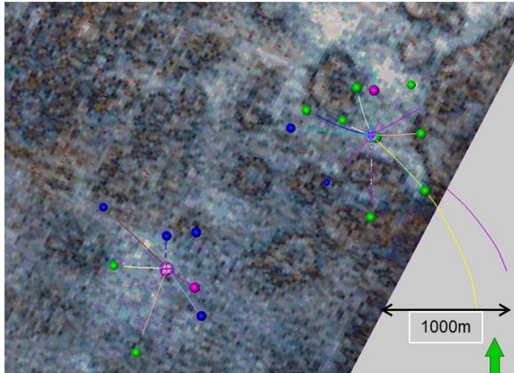
Figure 6: Diffraction imaging with edge enhancement and drilling mud loss data. Blue represents partial losses, green is complete and purple is no losses.
