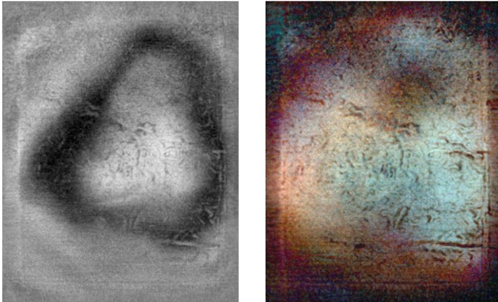
Figure 4: Before (left) and after (right) edge enhancement using frequency decomposition and color blending of diffraction imaged data for fault and fracture zone detection in the reservoir
