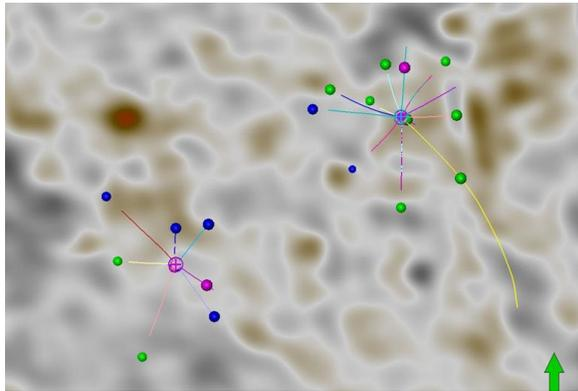
Figure 7: Reflection imaging with drilling mud loss data. Blue represents partial losses, green is complete and purple is no losses.
