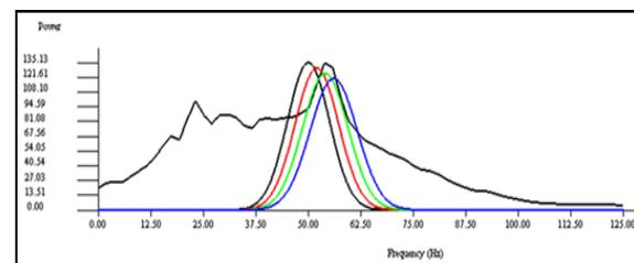
Figure 1: Spectral decomposition for shallow collapse features. The color of the frequency distribution curve indicates the RGB component for the color blend. The frequency magnitude of the shallow section is the black curve displayed in background.
